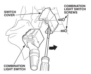
8. Using a flat-tip screwdriver wrapped with electrical tape, lift the switch cover slightly, then remove the switch, and discard it.
