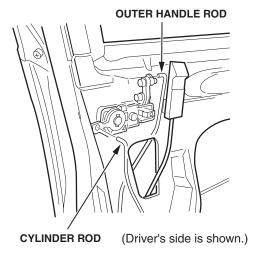
7. Pull down on the retainer clip with a hook-shaped tool. Remove the lock cylinder.
