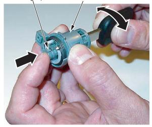
13. Using your thumb and forefinger to hold the tumblers, remove the key from the inner cylinder, being careful not to drop any tumblers and springs.
