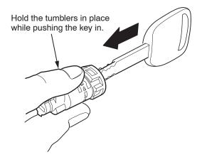
16. Leave the key in the cylinder. Reinstall the plastic retainer and spring if you removed them in step 10. Hold the plastic retainer and spring on the housing, and insert the inner cylinder. Rotate it left and right to engage the spring to the inner cylinder. Make sure the spring is properly seated to the inner cylinder.
