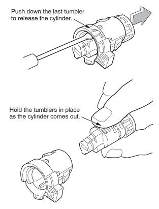
12. While turning the key left and right and pushing on the rear of the inner cylinder to release the spring, slowly remove the cylinder from the housing.
