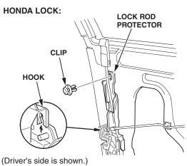
6. Disconnect the outer handle rod and cylinder rod.
