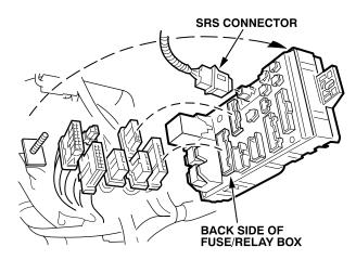
7. Pry away the four tabs, then use a flat-tip screwdriver to remove the multiplex control unit from the fuse/relay box.
