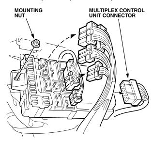
Unplug the electrical connectors from the back of the fuse/relay box. Remove the box from the vehicle.
