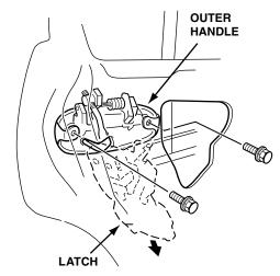
4. Pull the outer handle away from the door. Do not disconnect the outer handle rod. Place a shop towel in the door handle opening to protect the door from getting scratched.
