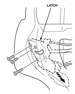
3. Pull the latch assembly down, and remove the door handle mounting bolts.
